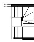
Partial Main Floor Plan with Optional Finished Stair to Basement with Opening (Adds 0 Sq. Ft. to Main Floor; Must Add 58 Sq. Ft. of Finished Basement Area Minimum)
