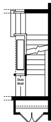
Partial Main Floor Plan with Optional Finished Stair to Basement (Adds 0 Sq. Ft. to Main Floor)
